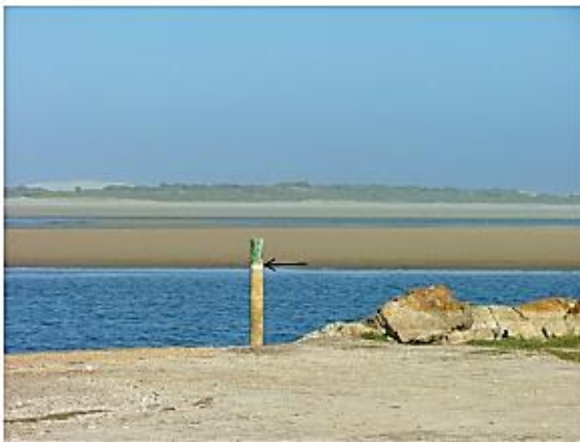
Photo 29: The beacon at Prawn Flats, which is intended to inform artificial breaching of the estuary (when the water level reaches a minimum of 2.1 m above mean sea level [arrow]).
