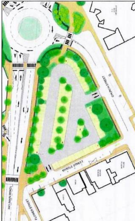
Figure 27: Church Street Parking Area Conceptual Design [Refer to Appendix F for a larger print]
