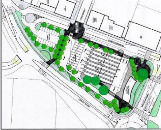
Figure 26: Hermanus CBD Taxi Rank Conceptual Design [Refer to Appendix E for a larger print]
