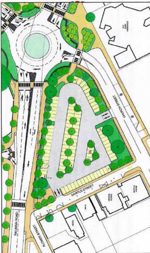
Figure 22: Church Street Parking Area Conceptual Design [Refer to Appendix F for a larger print]
