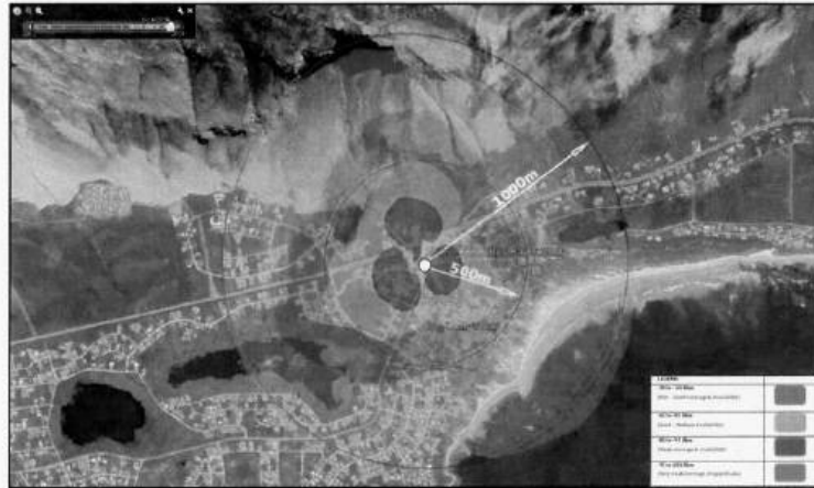
Fig. 12 – RF plot indicating the expected increase in coverage provided by the proposed installation (Source: As composed by the client's RF Planners)
