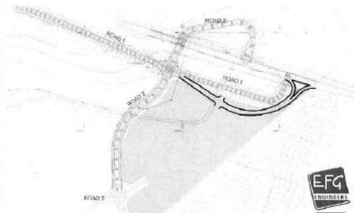
Figure 23: Road design proposal for the new access via an interchange from the R43 Provincial Road
