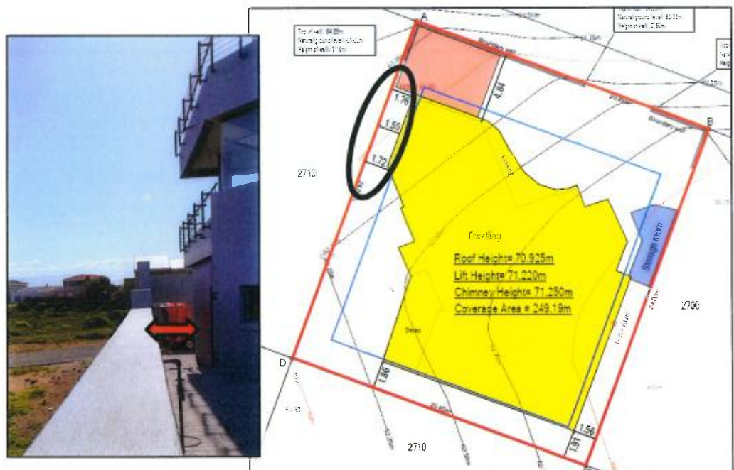
Figure 13: Western Building Line Departure
