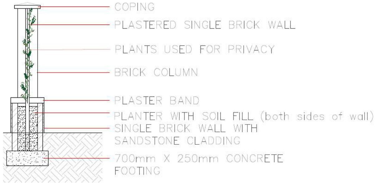
Figure 10: Typical Detail: Boundary Wall (no date) Source: WRAP Town Planning & Project Management
