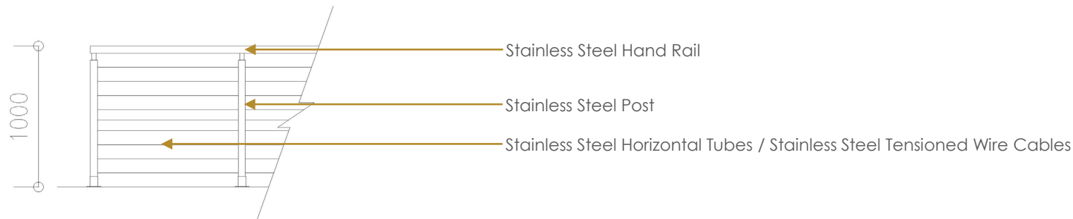
Typical Balustrade Elevation
