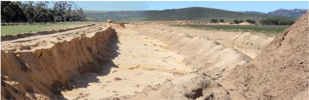
Photo 13: Sand Mining Method Indicating Sand Excavation and Topsoil Berms
