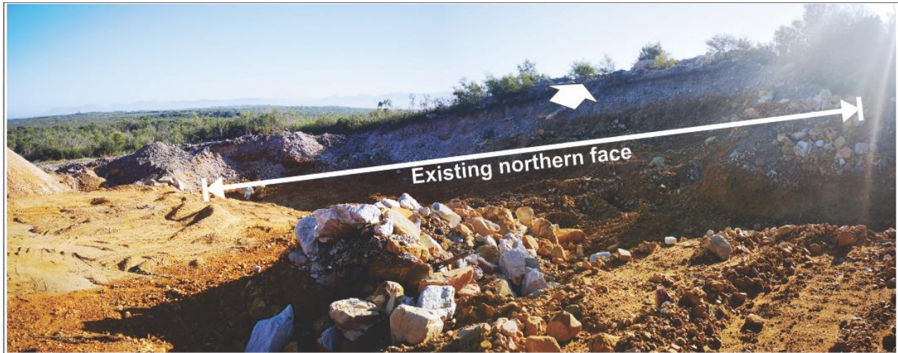
Photo 11: Existing northern face of gravel quarry. Note that this face has not yet reached its final position in terms of the existing mining permit, but the plan is to further advance it northwards as part of the Section 102 application.
