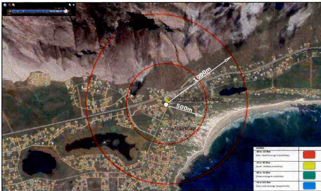
Fig. 11 – RF plot indicating coverage provided by existing telecommunication infrastructure within a 500m and 1000m radius (Source: As composed by the client's RF Planners)
