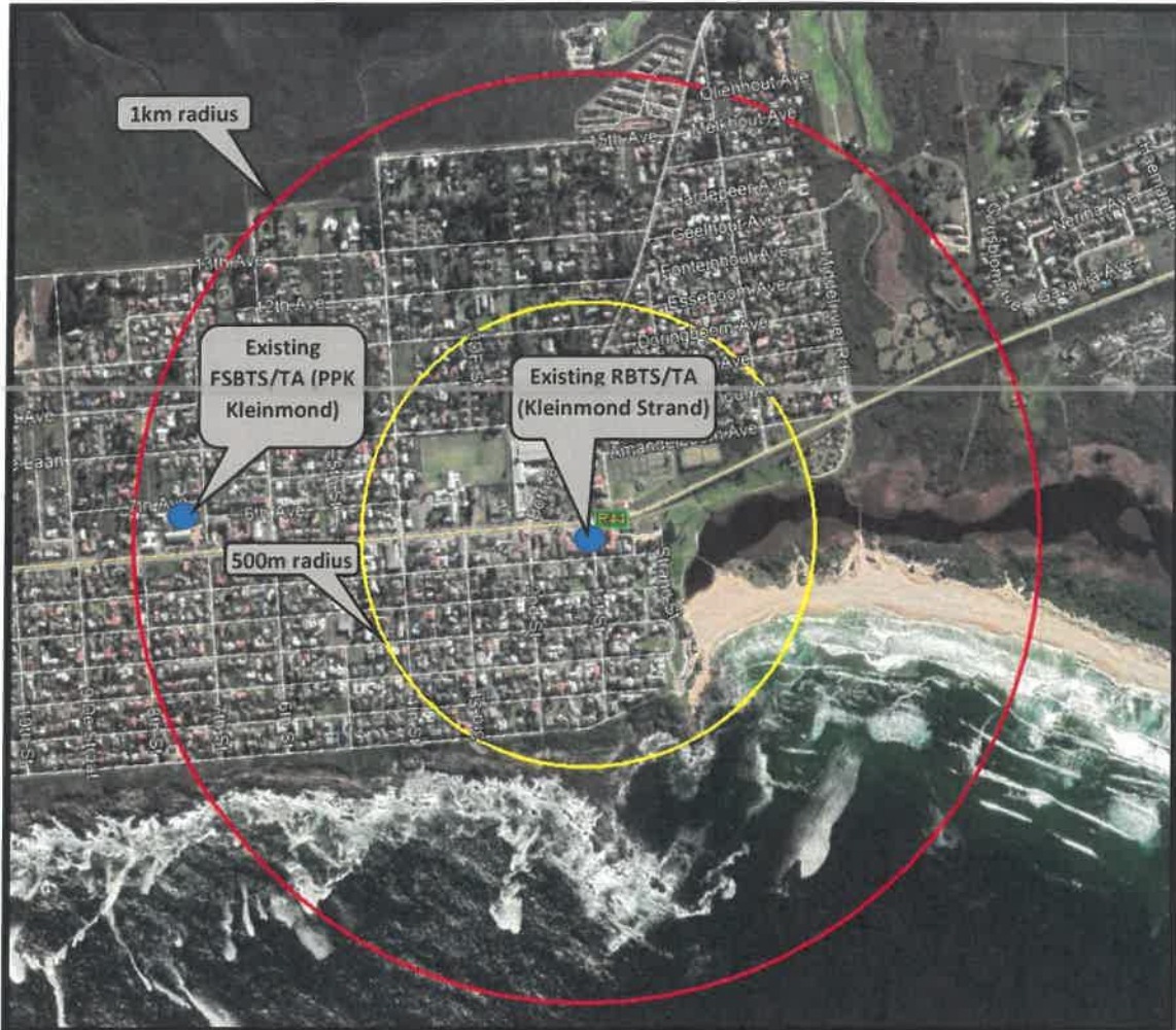
Figure 12 - 500m and 1km radius of the existing site and surrounding base stations
