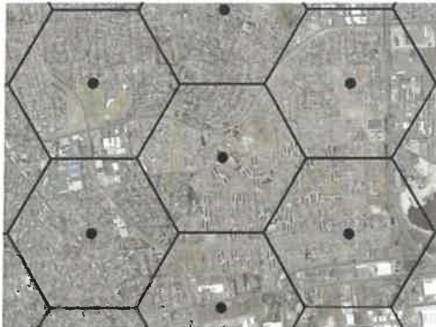
Figure 9 - Initial Coverage (Cell) provided by Telecommunication Base Stations
