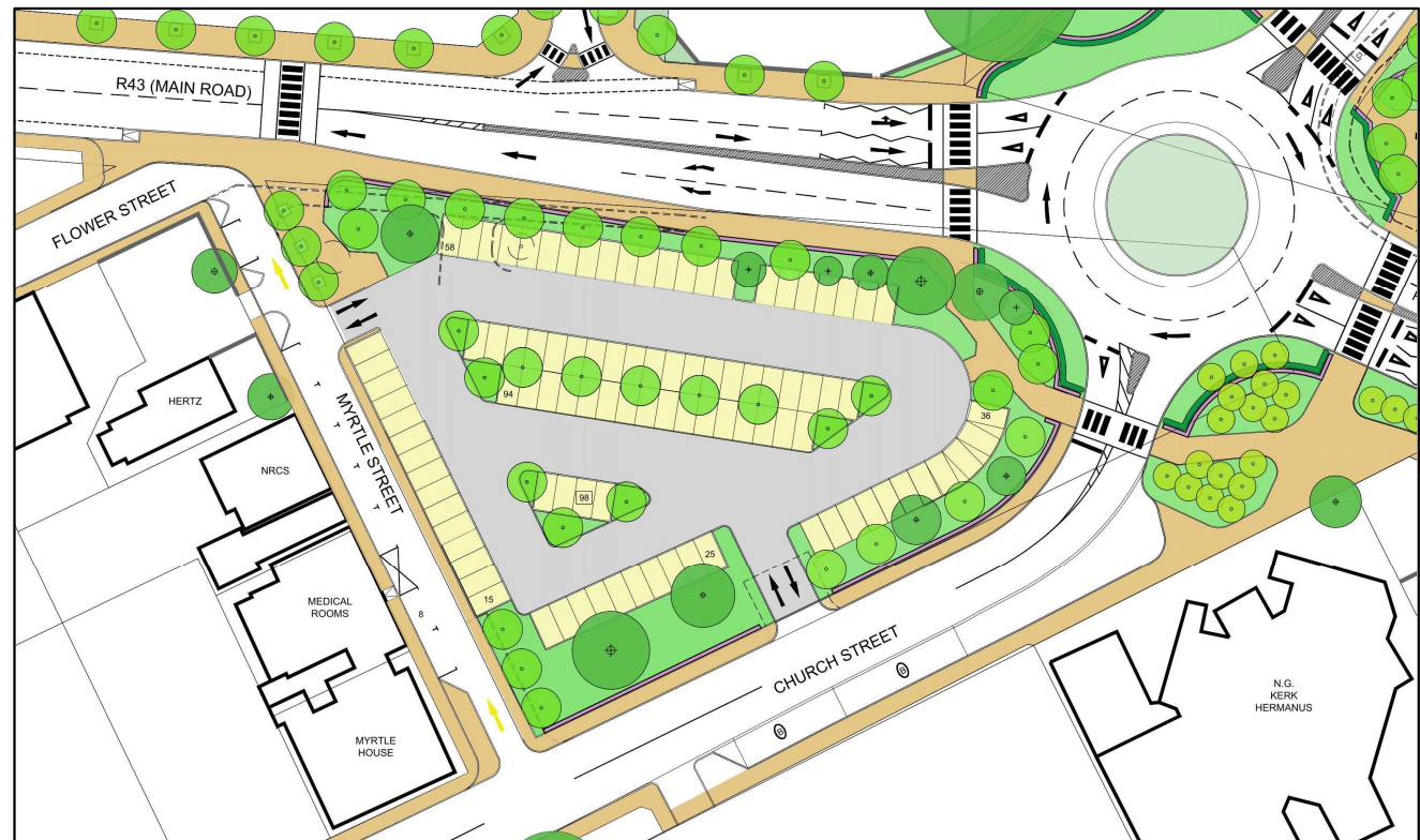
Figure 22: Church Street Parking Area Conceptual Design [Refer to Appendix F for a larger print]
