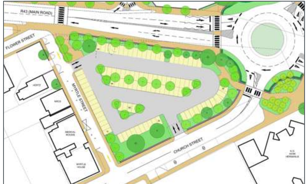
Figure 27: Church Street Parking Area Conceptual Design [Refer to Appendix F for a larger print]
