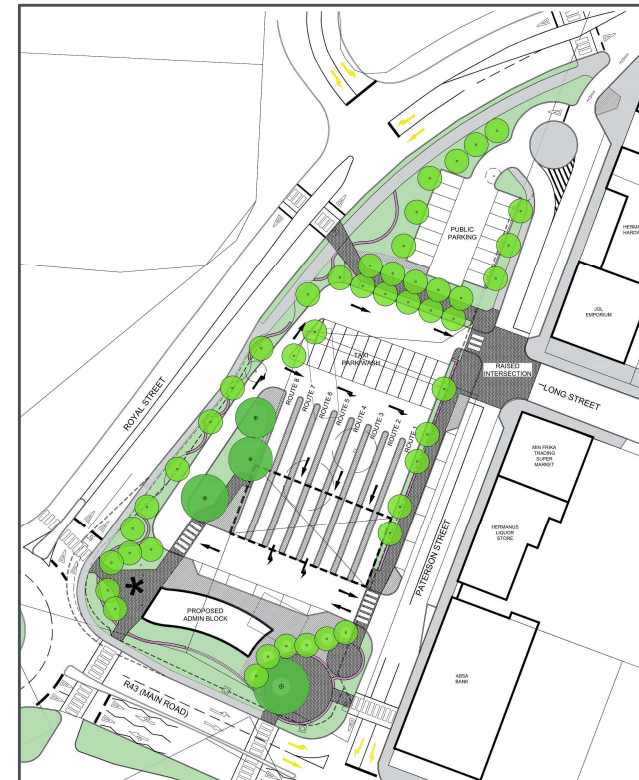
Figure 26: Hermanus CBD Taxi Rank Conceptual Design [Refer to Appendix E for a larger print]
