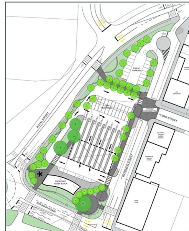
Figure 21: Hermanus CBD Taxi Rank Conceptual Design [Refer to Appendix E for a larger print]
