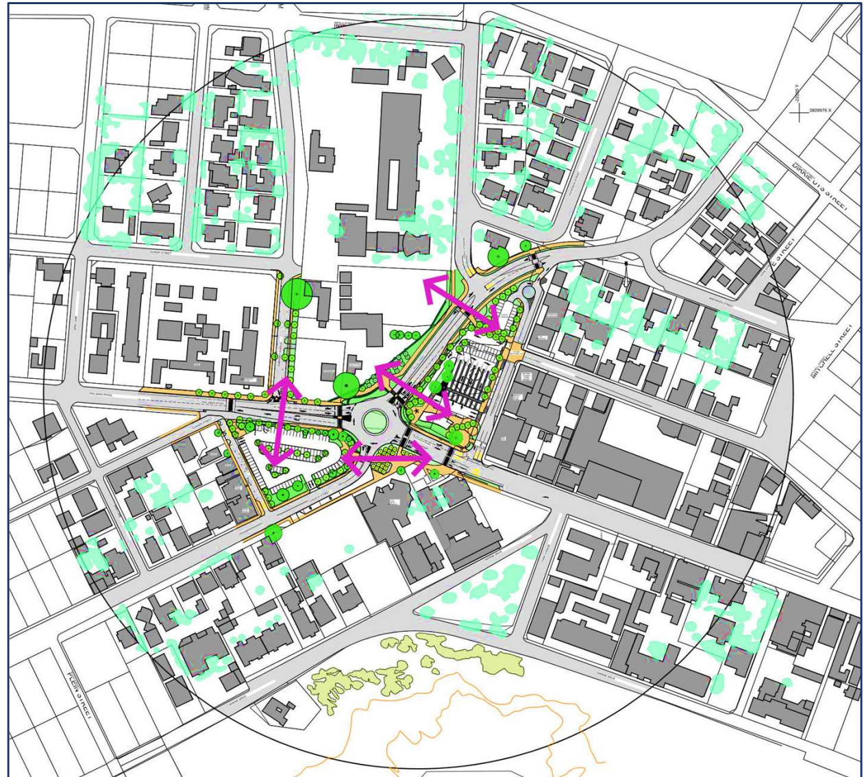
Figure 25: Dominant pedestrian movement patterns taken into consideration when creating safe and accessible spaces
