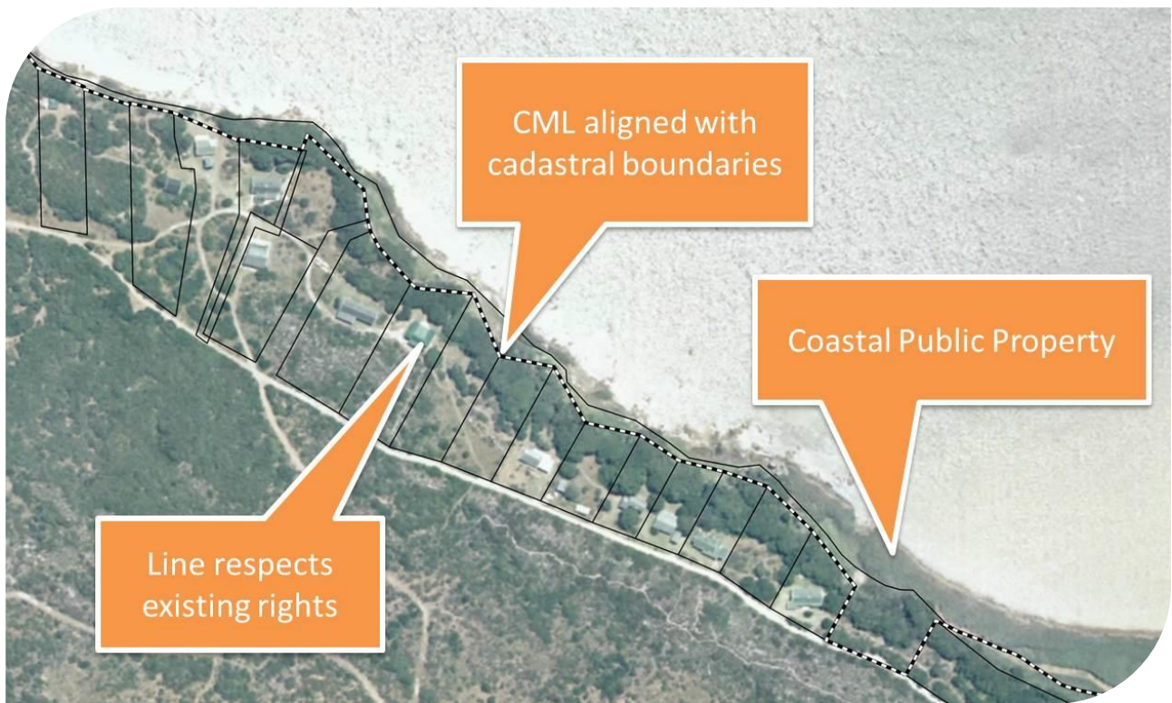
Figure 9: Example of the location of the coastal management (set-back) line in developed parts of estuaries
