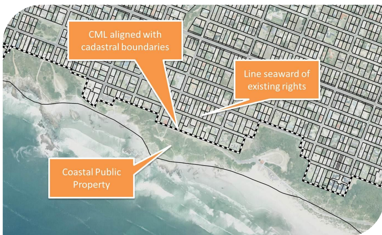
Figure 8: Example of the location of the coastal management (set-back) line in urban areas
