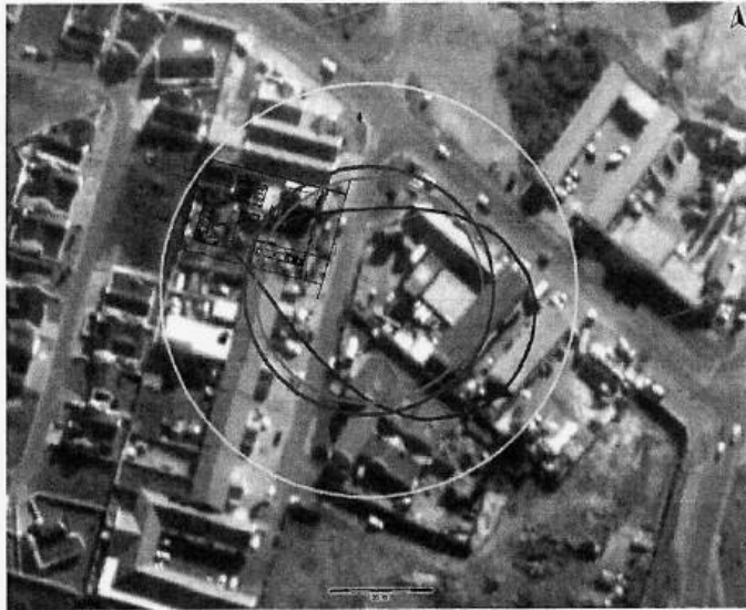
Flash Fire from a Catastrophic Leak at the Bulk Vessel
