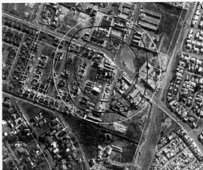
VCE from a Catastrophic Failure of the Proposed LPG Tanker Area
